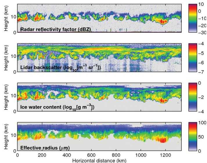
Figure 1. (Top two panels) CloudSat and CALIPSO observations of ice cloud over the Indian Ocean on 17 July 2006; (bottom two panels) ice water content and effective radius retrieved by the variational algorithm of Delano and Hogan (2008).
