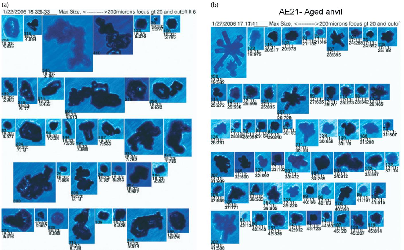
Figure 2. Images of ice crystals detected by Manchester University's Cloud Particle Imager mounted on the Airborne Research Australia's Egret Aircraft flying in anvils from Hector clouds over the Tiwi islands. (a) Crystals characteristic of those close into the main convective cell with large irregular crystals and aggregates including chain aggregates. (b) Crystals characteristic of an aged anvil featuring bullet rosette type crystals and small irregular crystals.
