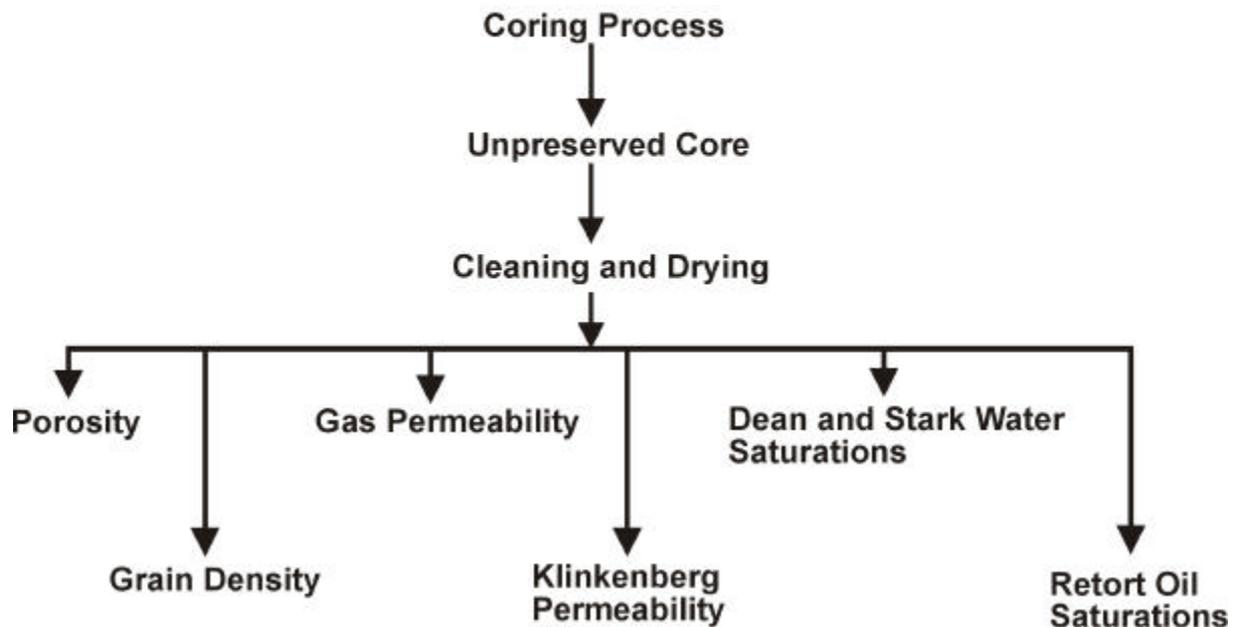
Each of the RCAL measurements made is discussed in detail, covering; the theory, test methods, and limitations of alternative methods. The topics covered will include:
