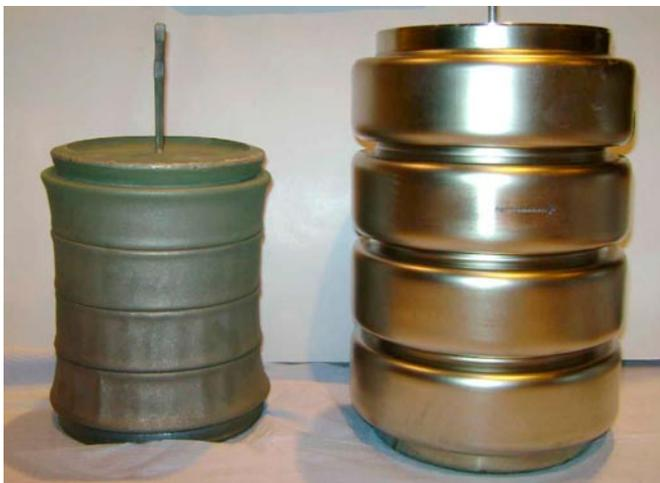
Figure 1: Pilot scale HIP cans before (right) and after (left) consolidation
