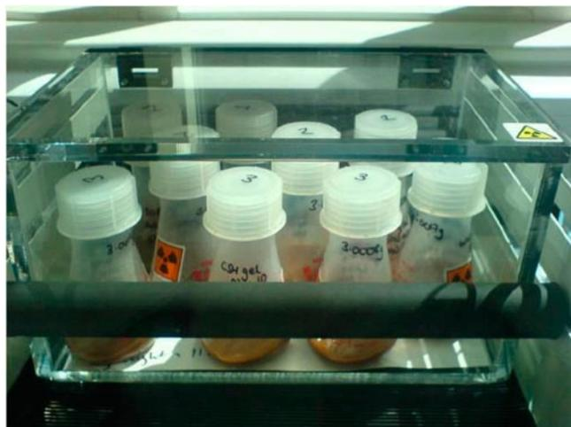
Figure 1: Batch experiment setup used in this study. Experiments used  $^{90}\text{Sr}$  tracer to measure Sr sorption
