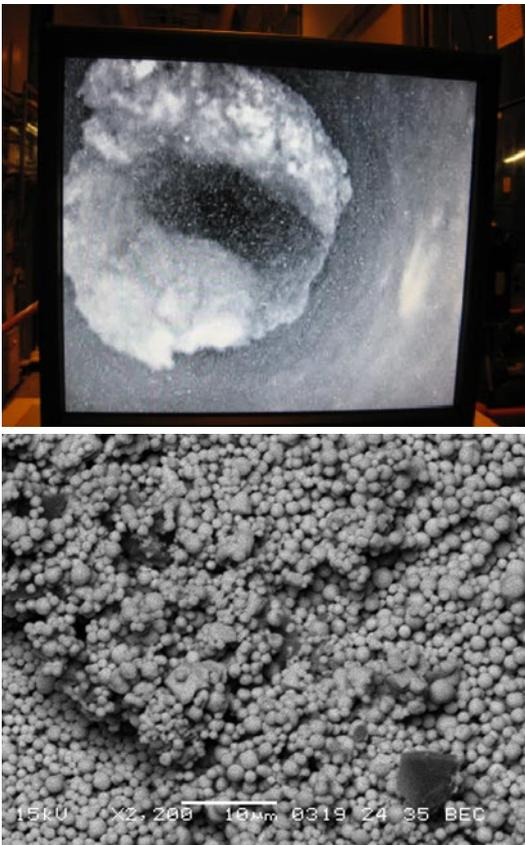
Figure 8: Endoscope image of the  $\text{CsTcO}_4$  blockage in the WVP dust scrubber-condenser pipework (top) & backscattered SEM image of agglomerated  $\text{CsReO}_4$  particles in the VTR pipework (bottom)
