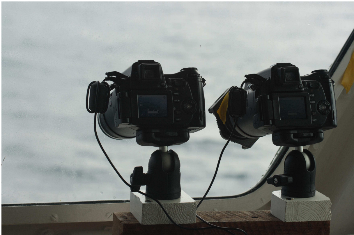
Figure 28.1 Digital cameras installed on the port side of the bridge to take images of the sea surface abeam of the ship.
