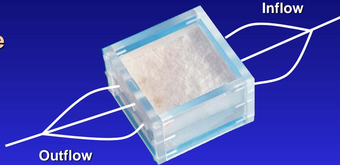
Flow manifolds at input & output ports
