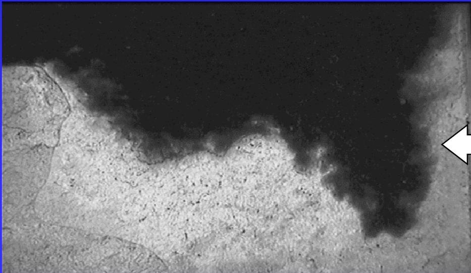
Clear water is replaced by dyed water in the flow through a rough fracture
