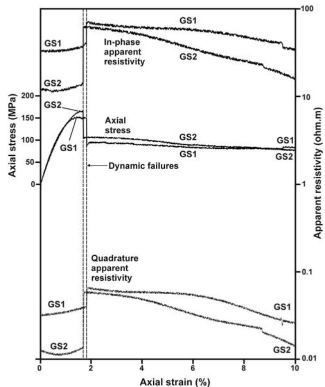
**Figure 6.** Experimentally determined axial stress and in-phase apparent electrical resistivity at 1 kHz as a function of axial strain during the progressive axial deformation of two samples of carbon-bearing graphite schist. GS1 3.1% wt/wt carbon, GS2 7.37% wt/wt carbon.
