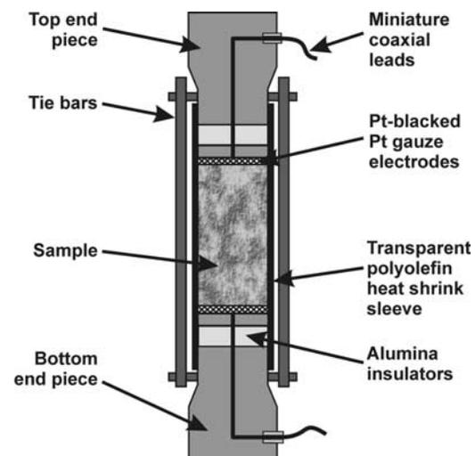
**Figure 4.** Diagrammatic representation of the experimental assembly showing the axial electrical measurements.
