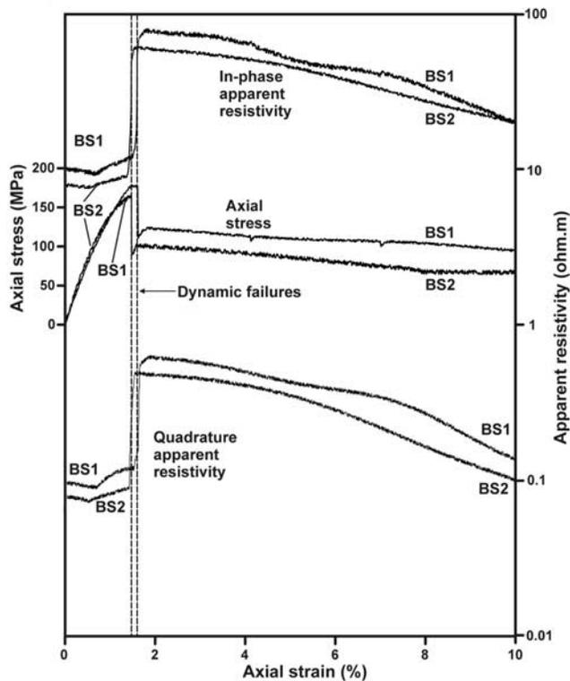
**Figure 5.** Experimentally determined axial stress and in-phase apparent electrical resistivity at 1 kHz as a function of axial strain during the progressive axial deformation of two samples of carbon-bearing black shale. BS1 8.12% wt/wt carbon, BS2 10.06% wt/wt carbon.
