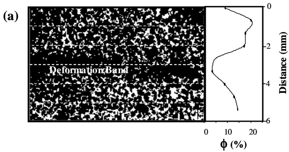
**Figure 3.** Thin-section image analysis porosity of deformation band and host rock
