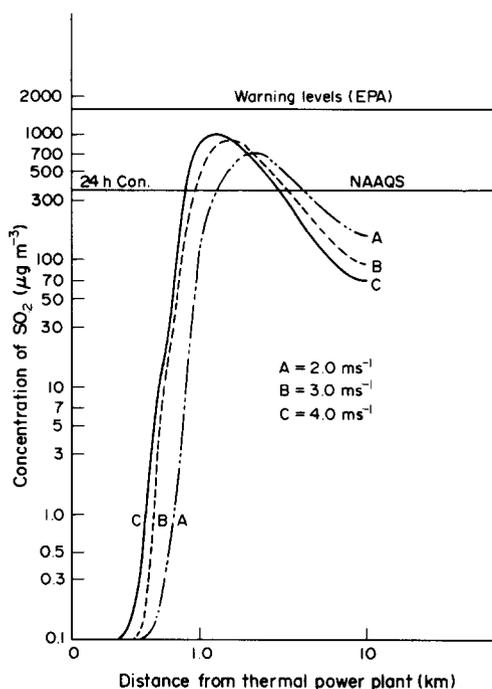
Fig. 4. Computed concentration of SO<sub>2</sub> for downwind distances from the thermal power plant for wind speeds of 2, 3 and 4 m s<sup>-1</sup>.
