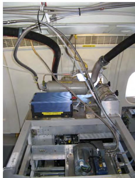
(b) WAS sample pumps and pressure reliefs located in the aircraft main cabin.
