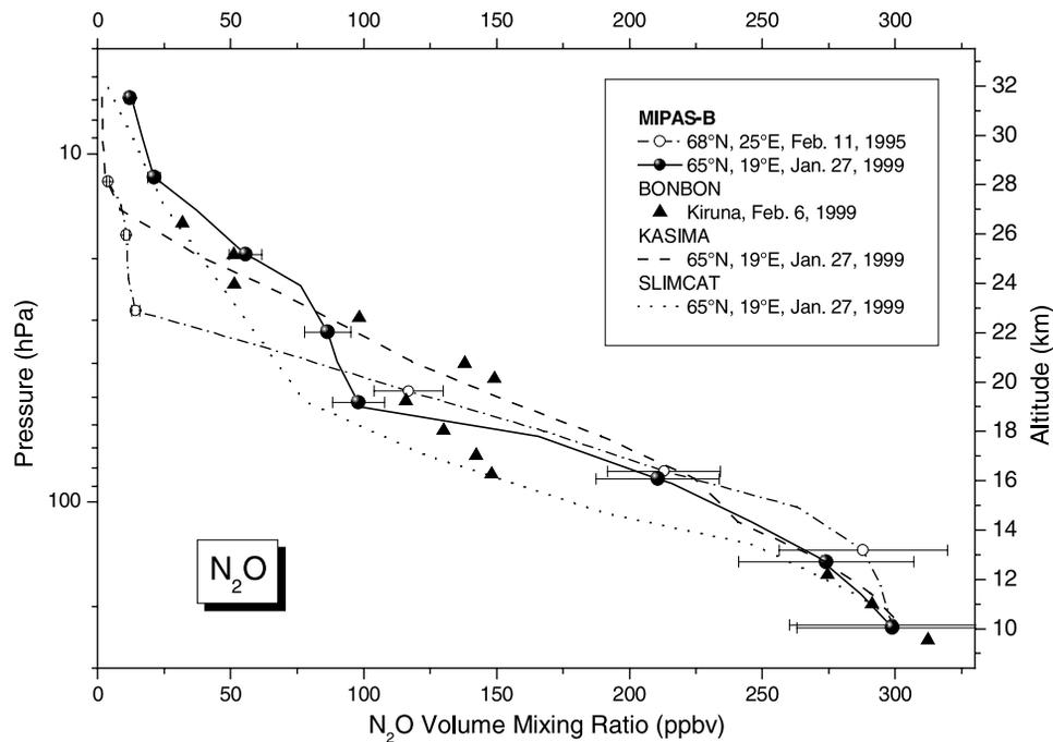
**Figure 2.** N<sub>2</sub>O volume mixing ratios measured by MIPAS-B on 27 January 1999 (solid line with symbols) and modeled by KASIMA (dashed line) and SLIMCAT (dotted line). An in situ observation (BONBON) [Müller *et al.*, 2000] 9 days after the MIPAS flight shows a similar characteristic of the air masses. For comparison a MIPAS N<sub>2</sub>O profile measured well inside the polar vortex on February 11, 1995 is shown, too.
