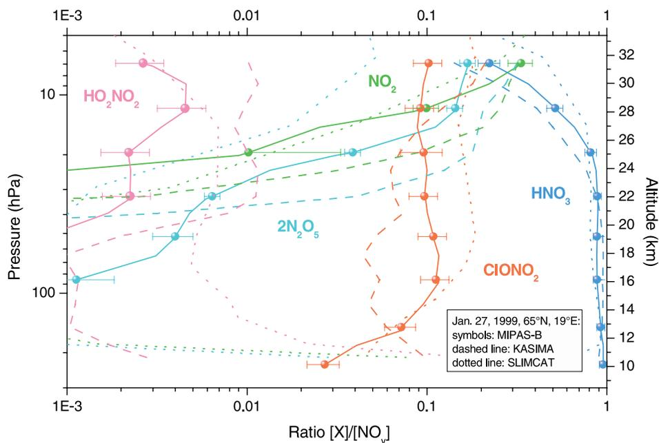
**Figure 6.** Comparison of the ratios of the individual NO<sub>y</sub> components on 27 January 1999 (solid lines with symbols) compared to SLIMCAT (dotted lines) and KASIMA (dashed lines).
