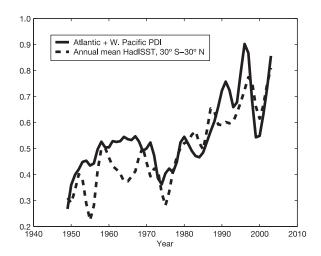
Figure 3 | Annually accumulated PDI for the western North Pacific and North Atlantic, compared to annually averaged SST. The PDI has been multiplied by a factor of  $5.8 \times 10^{-13}$  and the HadISST (with a constant offset) is averaged between 30° S and 30° N. Both quantities have been smoothed twice using equation (3). This combined PDI has nearly doubled over the past 30 yr.
