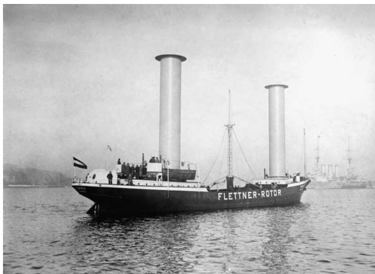
Figure 5. Anton Flettner's first rotor ship, the Baden-Baden, crossed the Atlantic in 1926.
