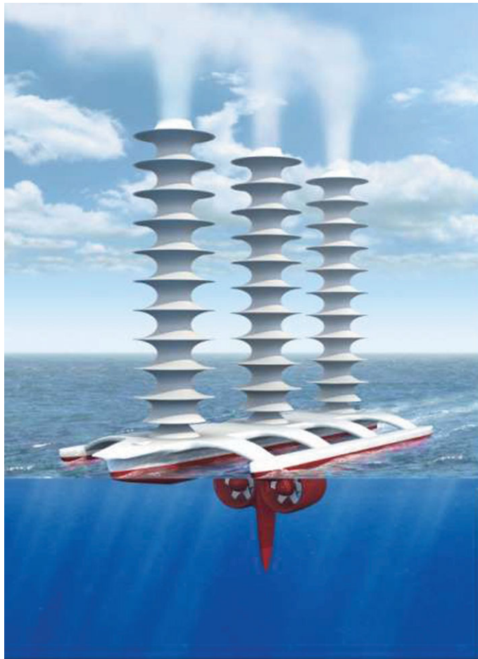
Figure 9. Artist's impression of a Flettner rotor ship. Reproduced from Gadian et al. [51]. (Online version in colour.)
