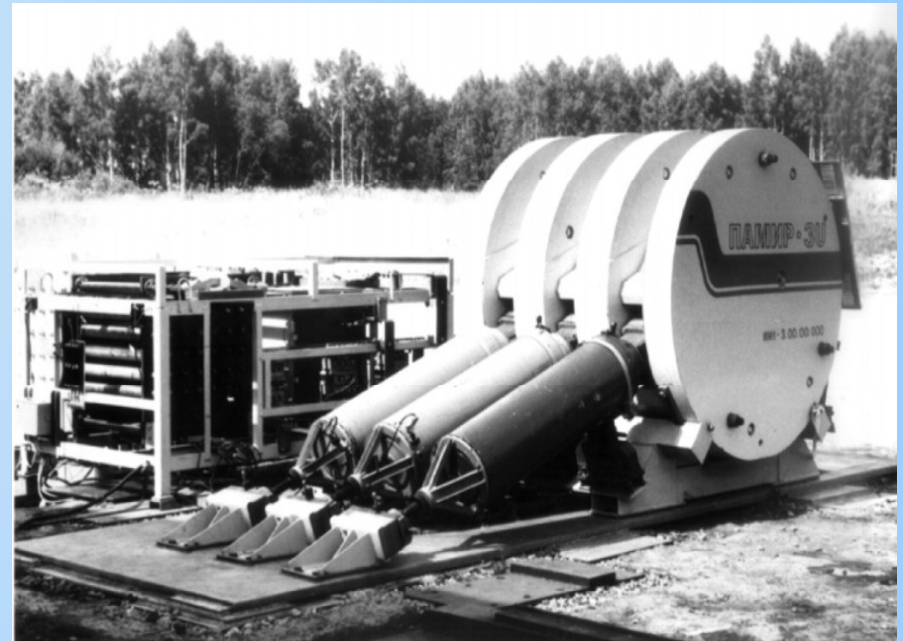
Pamir 3U 15 MW pulsed MHD generator at the Kyrgyzstan site.
