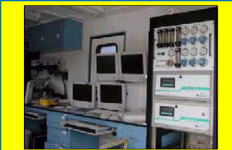
Cuttings gas measurement (Haliburton) is routinely carried out on site as the well is drilled.
