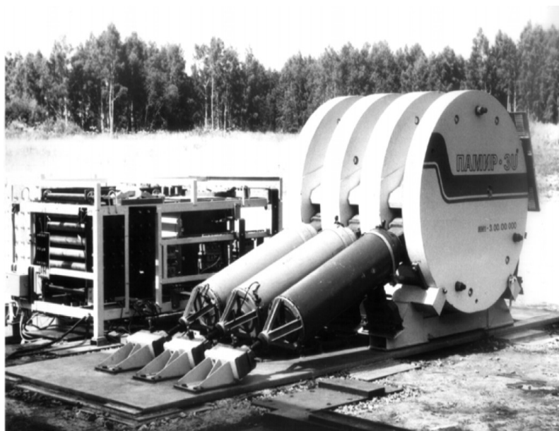
A 1500 MA pulsed MHD generator at the Kyrgyzstan site.
