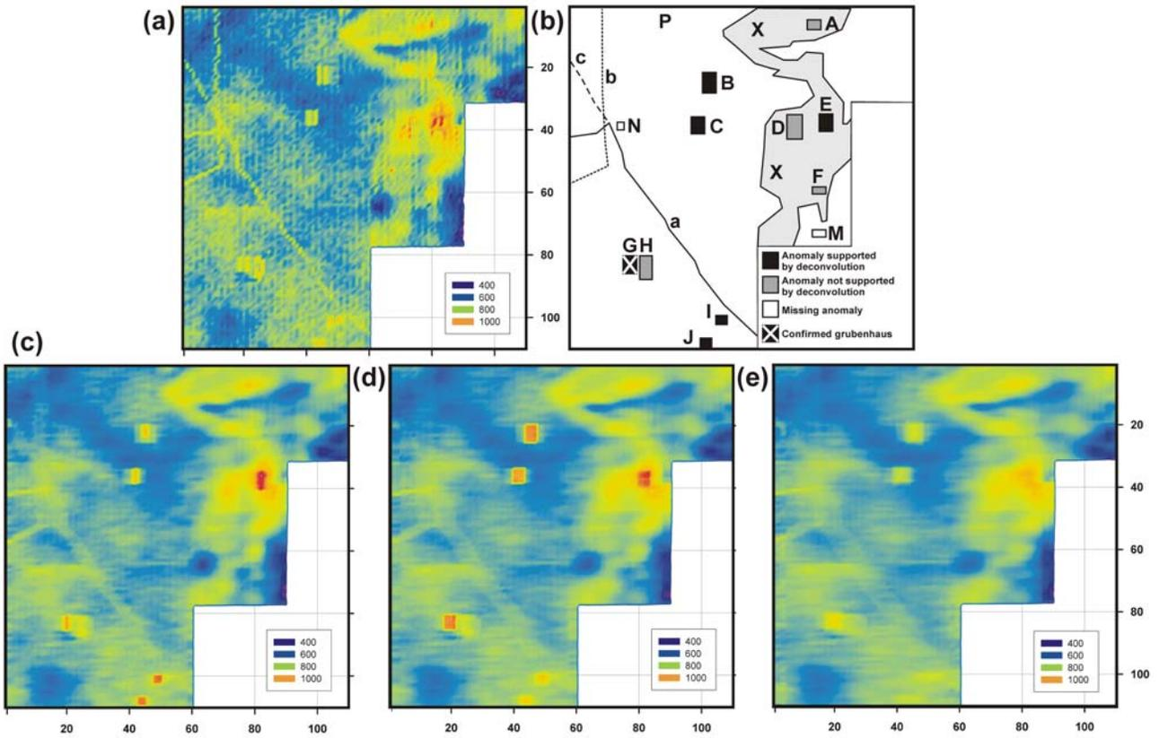
**Figure 2.** Resistivity maps of the survey area before and after digital filtering. (a) Raw resistivity data. (b) Initial interpretation. (c) Data deconvolved with a source signature of width  $w = 3$  m, depth  $d = 0.5$  m, and a topsoil cover of  $h = 0.3$  m, (d)  $w = 4$  m,  $d = 0.5$  m and  $h = 0.3$  m, (e)  $w = 5$  m,  $d = 0.5$  m and  $h = 0.3$  m.
