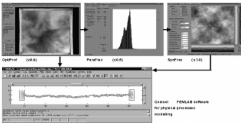
**Figure 2** The software framework for the full characterization of rough fractures in rocks. OPTIPROF provides considerable control over the imaging process and calculates the final surface topographies. This data can be input into FEMLAB physical process modelling software. Input also comes from numerical models created using PARAFRAC and SYNFRAC software, which are tuned to the profiling data.
