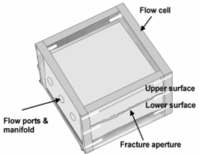
**Figure 9** Flow cell containing HFPMs for fluid flow experiments.
