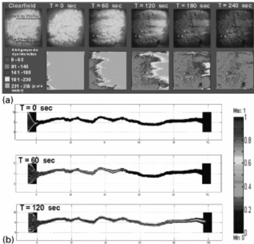
**Figure 10** A combined experimental-modelling approach for the tracking of fluid flow through rough fractures. (a) Experimental fluid flow through an HFPM of syenite for when  $Re = 1.2$ , Flow charge,  $Q = 0.08 \text{ cm}^3$  and (b) respective simulations. (c) Experimental fluid flow for when  $Re = 12.6$ , Flow charge,  $Q = 0.76 \text{ cm}^3$ , and respective simulations (d).
