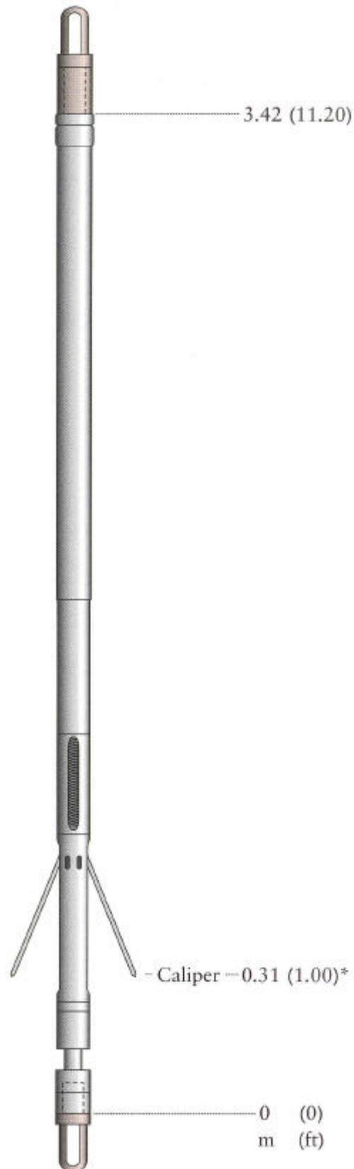
**Figure 9.1** The Reeves 2 arm caliper tool.
