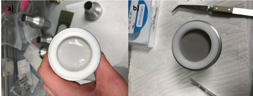
Figure S7: Filters before (a) and after sampling (b). The dark colour of the filter after ~1 hour sampling during the combustion event is clear. Filter sampling in Leeds during normal conditions does not yield dark filters.
