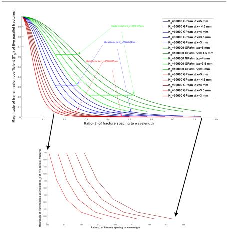
Fig. 11: Magnitude of transmission coefficient for 5 fractures  $|T_5|$  as a function of  $\xi$  for different values of normal stiffness  $K_n$  and fracture spacing  $\Delta x$  (the image has been modified from Parastatidis (2019)).
