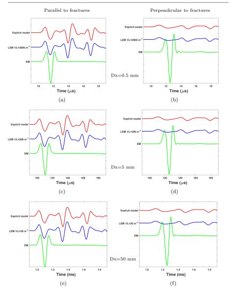
Fig. 10: Comparison of P-wave propagation parallel and perpendicular to the fractures for the Explicit, EM and the LEM (10a and 10b) the element size is 0.5mm and  $1/L=2000m^{-1}$ , (10c and 10d) element size is 5mm and  $1/L=200m^{-1}$  and (10e and 10f) element size is 50mm and  $1/L=20m^{-1}$  the explicit model consists of 5 fractures. It is clear from the waveforms that there is a linear connection between element size, maximum 1/L and maximum source frequency.
