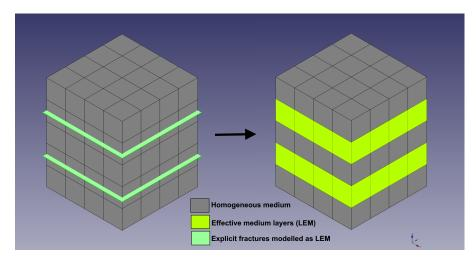
Fig. 1: The zones surrounding the predefined fracture positions are anisotropic while the rest are the background medium (as modified from Parastatidis (2019)). The finer the mesh of the model the thinner the LEM layer and the closer to the explicit model.
